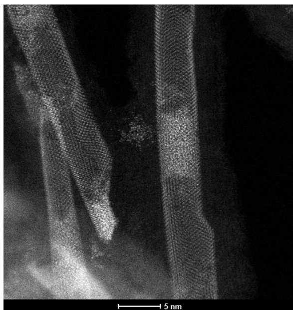
FIGURE 1. Aberration-corrected HAADF-STEM image showing a single-layered PbI 2 nanotube encapsulated within a multiwalled carbon nanotube
